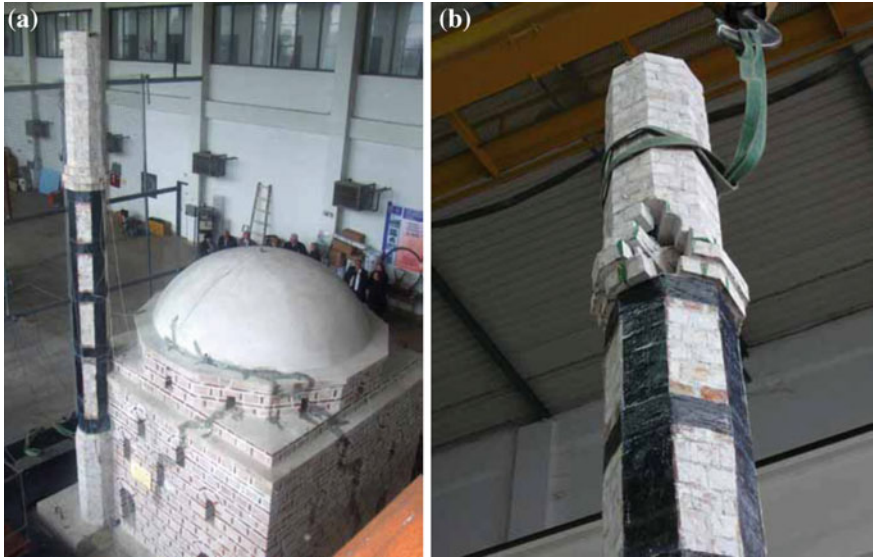
Fig. 4 The strengthened model of the mosque (a) and the collapse of the minaret (b)
