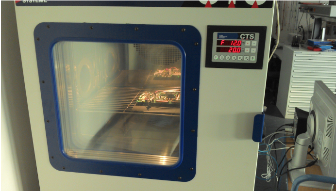
Fig. 5. The device under test inside the climate machine
