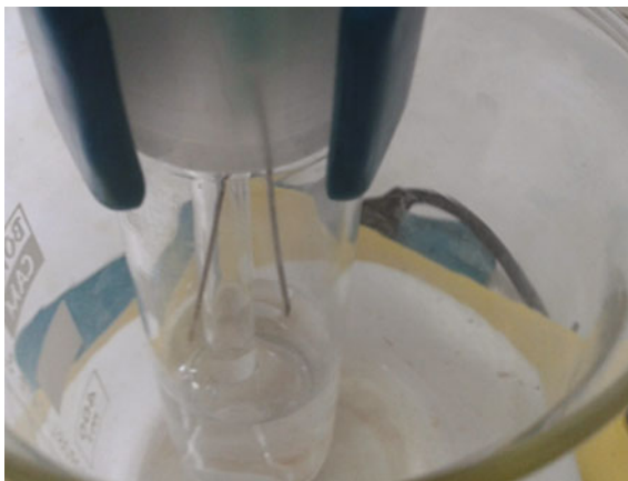
Fig. 18.3 Argon purging at the surface of the solution and inside the solution
