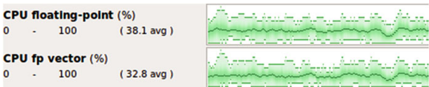
Fig. 10 32.8% mean CPU floating point vector instructions used by the pure MPI kernel
