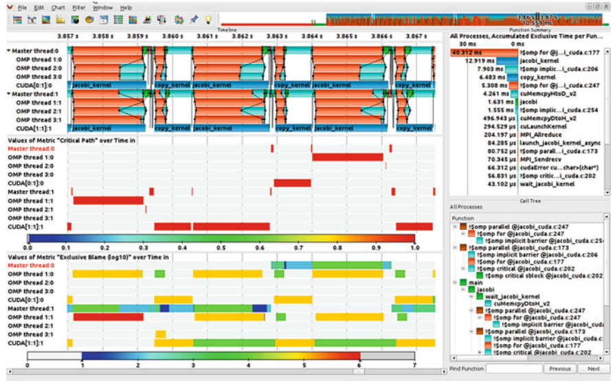
Fig. 4 Jacobi Method: Vampir screenshot for a scenario where the workload is almost equally balanced between CPU and CUDA device. The Master Timeline (top display) distinguishes activities according to the instrumentation. The Function Summary (top right display) shows the results of the hot-spot analysis (exclusive runtime) for each activity type. The Performance Radar (middle display) exposes the critical path (red), which changes between all available execution streams. The bottom Performance Radar uses color coding to illustrate the blame distribution
