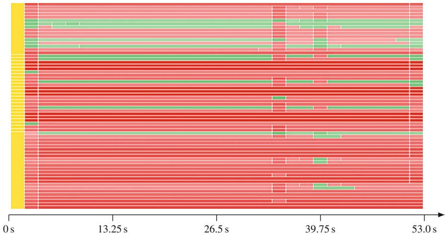
Fig. 5 Spatiotemporal overview of the application shown by Fig. 3. We still see the two temporal perturbations (around 35 and 40 s). State colors correspond to following the MPI calls: Yellow – MPI_Init, Green – MPI_Send, Red – MPI_Wait
