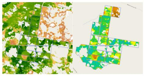
**Fig. 4.** Landsat 8 NDVI for the same day as is Fig. 3. The cloud mask is used the remove pixels which are determined to be invalid data (left). This image is then used to determine the crop coefficient (Kc) for cotton using a linear scaling (right).
