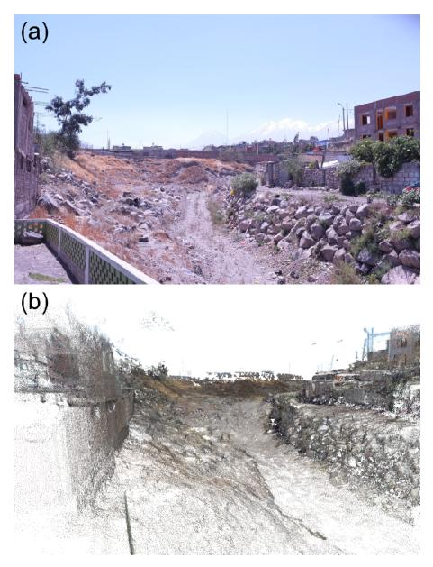
Fig. 2. (a) Case study area in Quebrada San Lazaro and, (b) dense point cloud reconstruction from the SfM-MVS
