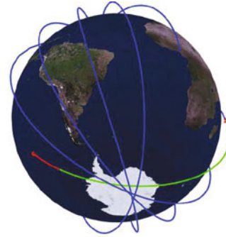
Figure 7. Re-entry simulation targeted towards the southern Pacific Ocean after solid rocket motor ignition
