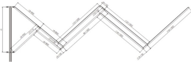
Figure 14. Final deployment mechanism dimensions in mm.
