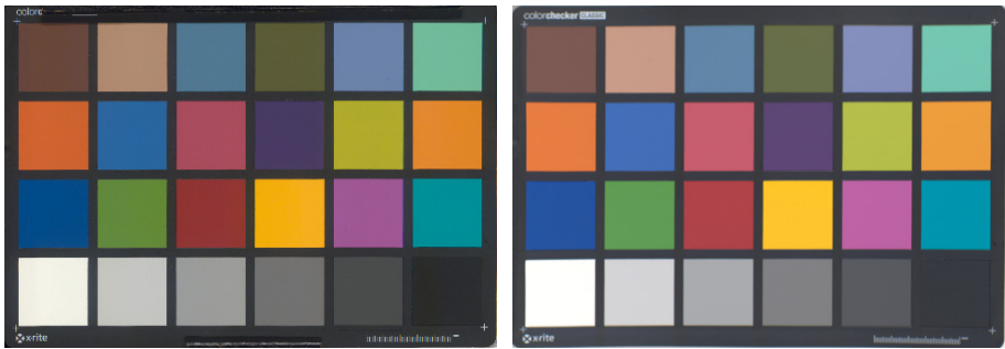
Fig. 1. RGB colour images of the X-Rite ® ColorChecker chart reconstructed from the hyper-spectral file-cube from IFAC-CNR (left) and IP-UEF (right)
