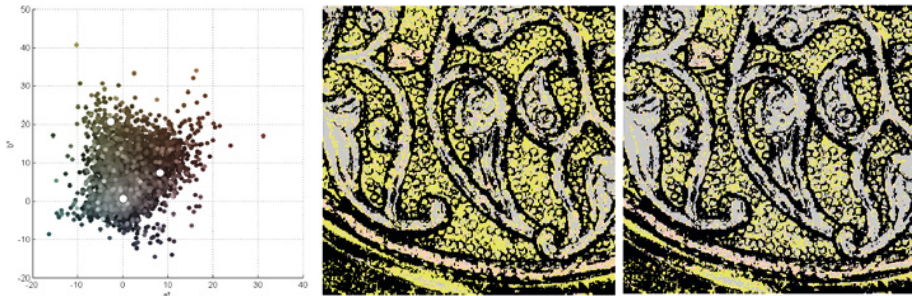
Fig. 17. (left) 10,000 pixels plotted on the CIELAB a^*-b^* chromatic plane, with centroids for the three metals; (centre) classification by hue angle; (right) classification by nearest colour
