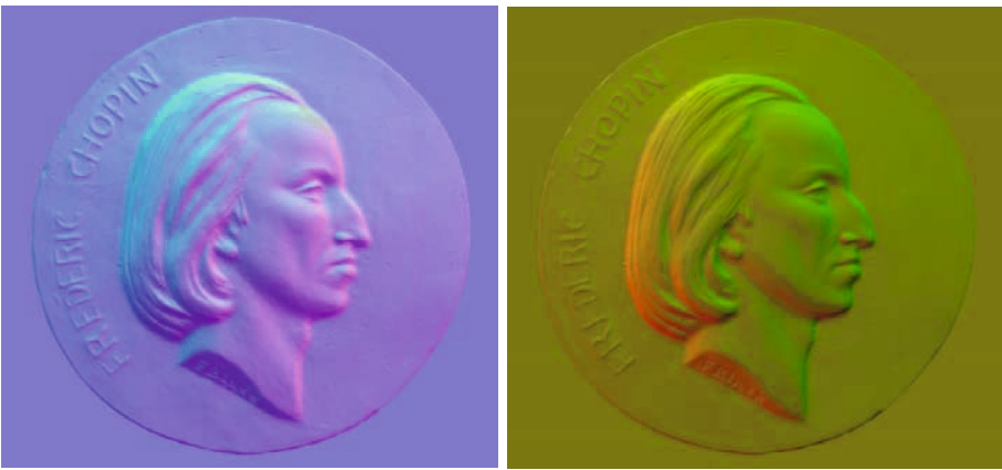
Fig. 6. (left) Photometric normal vectors in false colour (Nx red, Ny green, Nz blue); (right) False colour composite of gradients (P red, Q green)
