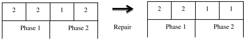
Fig. 3. Example of an initial chromosome for 2 compactors and 2 compaction fronts (left) and the final chromosome after the execution of the repair strategy (right)
