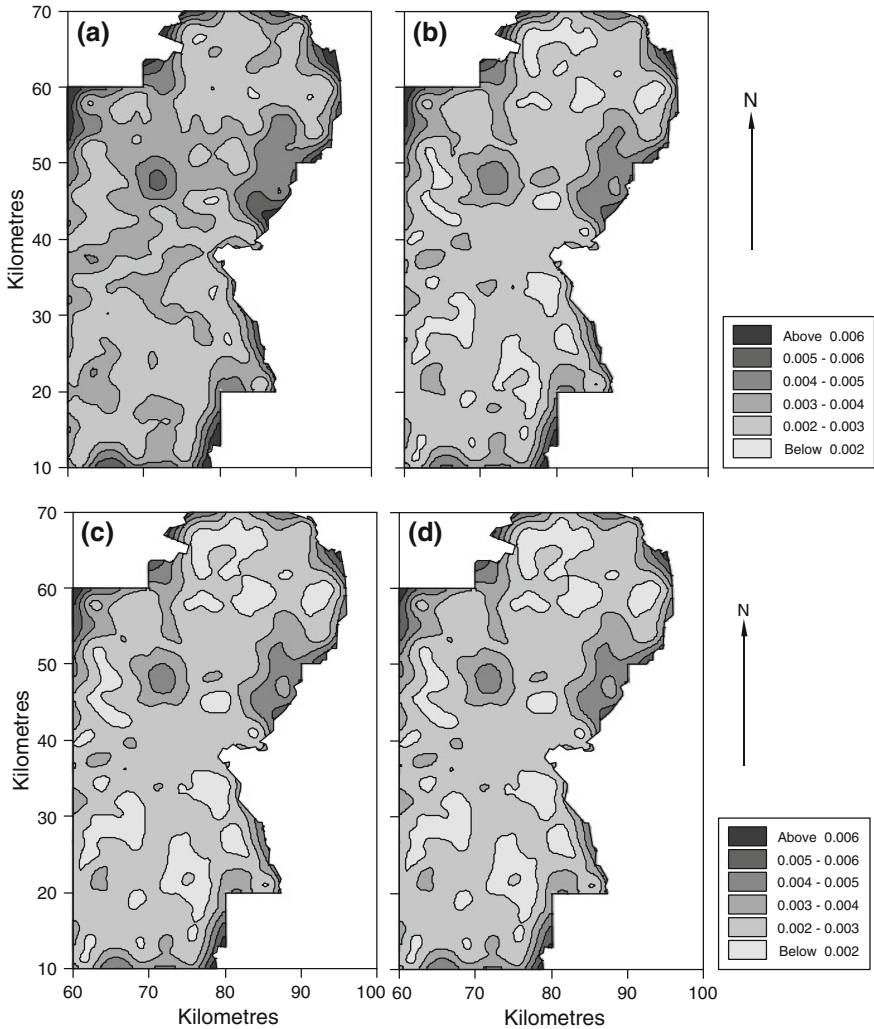
Fig. 4.7 Maps of ordinary punctual kriging variances of \log_{10}\text{Co} in the Borders Region of Scotland with the kriging neighbourhood set as follows: a 20 maximum points, 17 minimum points, b 40 maximum points, 37 minimum points, c 80 maximum points, 77 minimum points and d 140 maximum points, 137 minimum points
