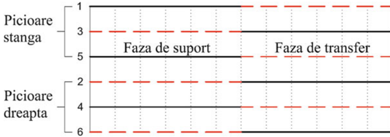
Fig. 14 Diagram of an alternating forward tripod gate
