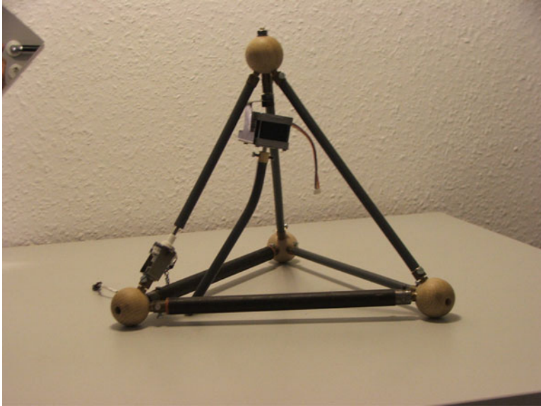
Fig. 13 The steering crawling tetrahedral mechanism
