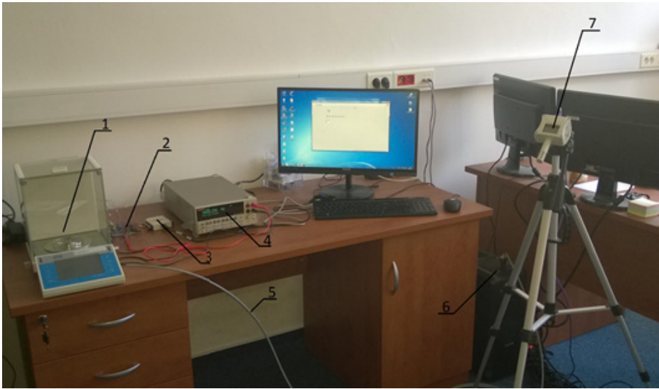
Fig. 4. Photo of the measuring stand: 1 – XA 82/220.3YA, 2 – micro-switches system, 3 – DAQ 6009, 4 – Keithley 2002, 5 – RS-232 cable, 6 – PC with LabVIEW software, 7 – thermo-hygro-barometer
