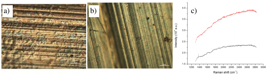
Fig. 8. Images of the surface of CuNi 2 Be bronze specimen: a) before the process, b) after the process, c) Raman spectra – absence of the graphene layer
