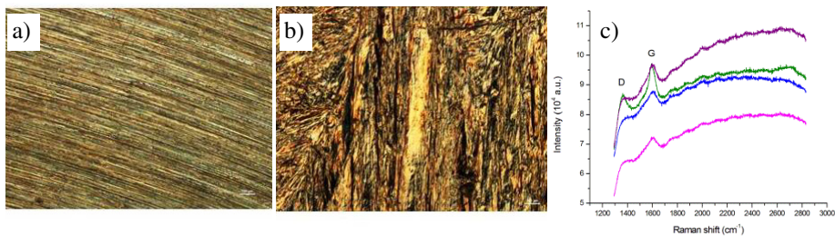
Fig. 7. Images of the surface of CuAl 6 Si 2 bronze specimen: a) before the process, b) after the process, c) Raman spectra – absence of the graphene layer
