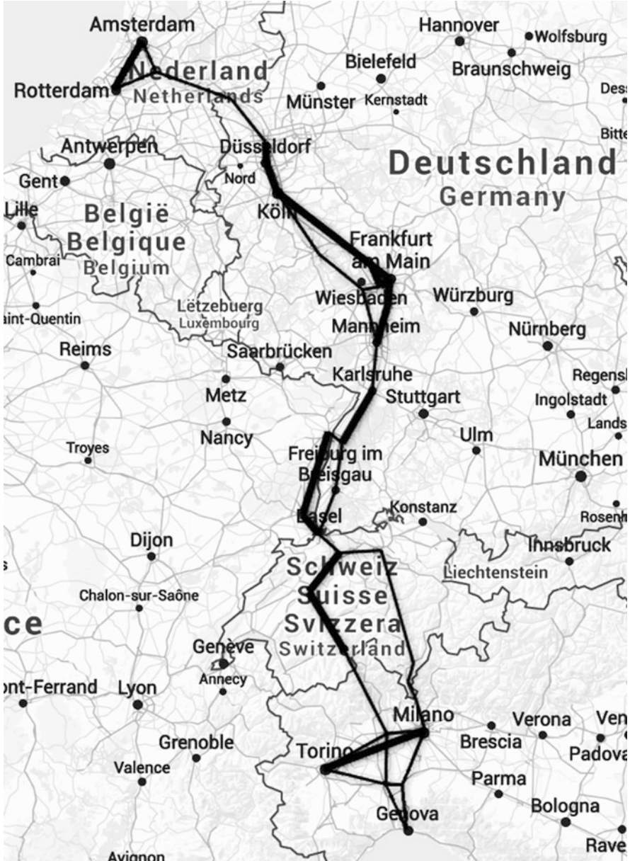
Fig. 3 Main rail lines along the corridor: thick links indicate lines allowing a speed over 200 kph, whereas thin links indicate lines with allowed speed not exceeding 200 kph. Source: CoDe24 Portal; base map: Google Maps, Google Inc.
