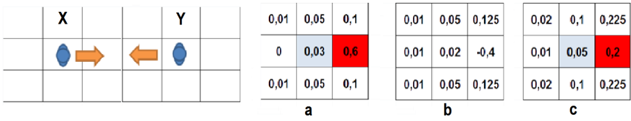
Fig. 6. Probability mask for determining best direction: individual probability for agent X (a), changing cell attraction mask for agent X from agent Y (b), result direction probability mask for agent X (c)
