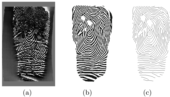
Fig. 1. Image pre-processing: (a) a low-quality fingerprint image, (b) the image after quality improvement, (c) the image after skeletonization
