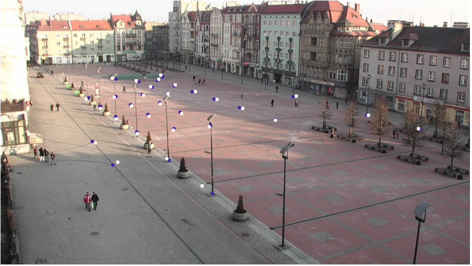
Fig. 4. Calibration results on exemplary dataset. Blue points were directly selected by the user. White points are world points (selected on the map) projected on the image plane using calculated intrinsic and extrinsic camera parameters.
