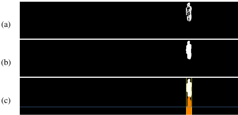
Fig. 5. The region, result from ego-motion compensation for moving object detection (a). Then, morphological process are performed on that region, the result is shown in (b) The histogram vertical projection is performed with specific threshold, so that the region of moving object is localized (c).
