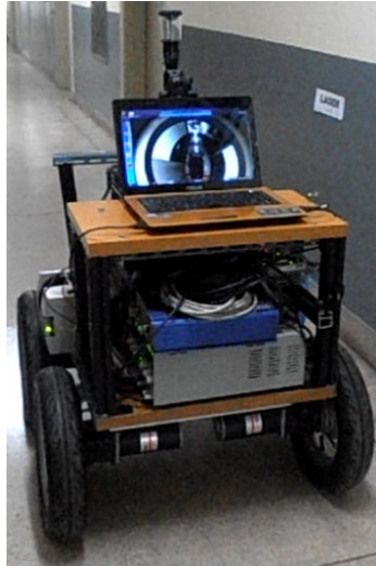
Fig. 2. An omnidirectional camera mounted on the mobile robot
