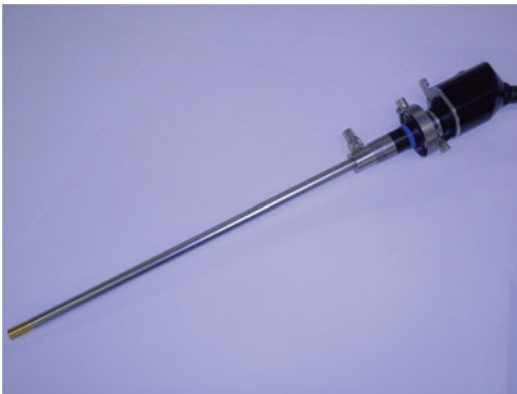
Fig. 25.2 New IRLS system. We developed a new IRLS system (OLYMPUS, Tokyo, Japan) for the detection of SN using both the absorption and the fluorescence imaging of ICG. One of the characteristics is instant switching of the observation mode between the absorption and the fluorescence imaging
