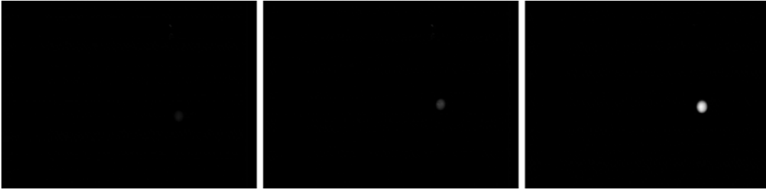
Fig. 37.2 Images of three different quantities of ICG, from left to right, 5, 10, and 100 pmol
