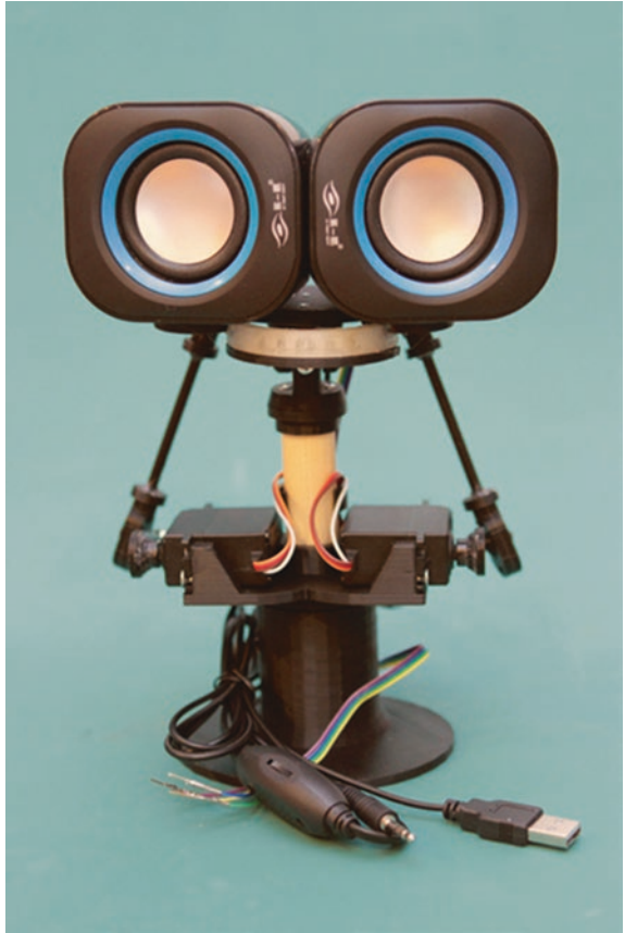
Fig. 8.3 3D printed animatronic robot head: an entry-level robotics/animatronics project by Adafruit, 2013–2014
