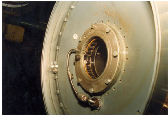
Fig. 2 Damaged elements of the aircraft engine middle bearing
