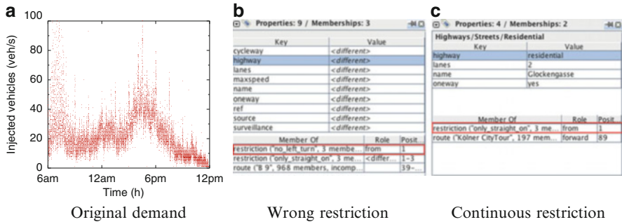
Fig. 11.7 Original data sources. (a) Volume of traffic injected in the road network between 6:00 a.m. and 12:00 p.m., according to the originalTAPASCologne origin-destination matrix. (b) Example of wrong restriction in OSM. (c) Example of continuous restriction in OSM (figure appeared in Uppoor et al. [44])
