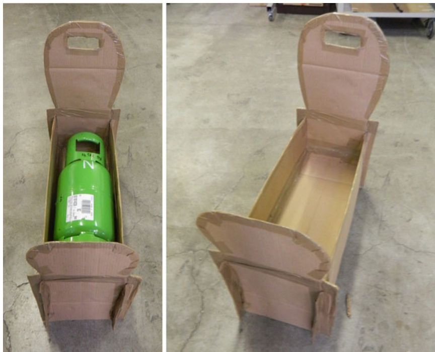
Fig. 10.3 Cardboard cradle prototype
