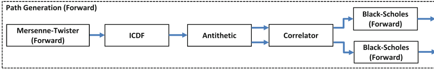
Fig. 7.5 Paths generation forward in detail, configured for two-dimensional American options
