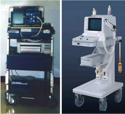
Fig. 2.4 The ADR-4000® and the Hitachi 405. Our references: two respectable collector machines, yet perfectly mobile to the bedside and able to achieve the ultrasound revolution since 1982 ( left ) and 1992 ( right ). Both are small in width ( left , 42 cm, right , 32 cm), and both have wheels, the key to the revolution. Please also see Fig. 2.2, showing how fine were these machines for developing lung ultrasound
