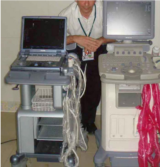
Fig. 37.3 Imagination: the fourth dimension. Mumbai, November 2008. Two machines from the same brand. The machine to our right ( dark screen ) is a laptop model (6 cm high). The left one is a traditional one (1 m high). Both have quite the same width. The laptop is even some cm larger, which means that in an emergency, the traditional machine would come faster at the bedside (thanks to the wheels). Laptop machines are a blessing for the warehousemen in ultrasound workshops, maybe their main interest
