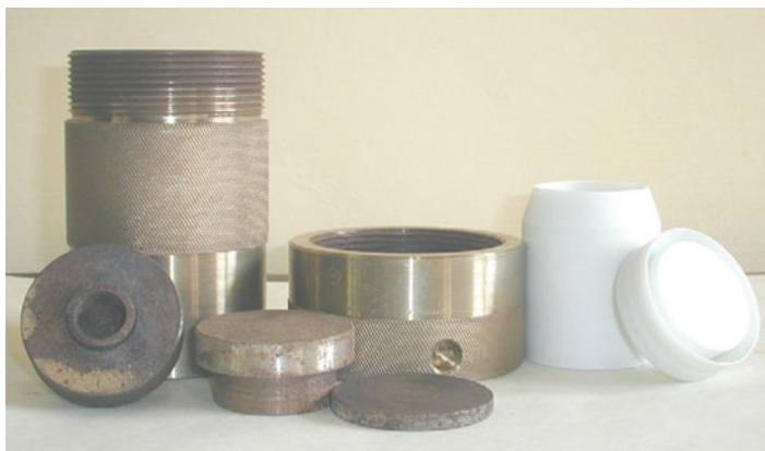
Fig. 1 A general-purpose hydrothermal autoclave. The hydrothermal reactions occur inside the Teflon container (Reproduced with permission from Byrappa and Adschiri [3]. Copyright 2007, Elsevier)
