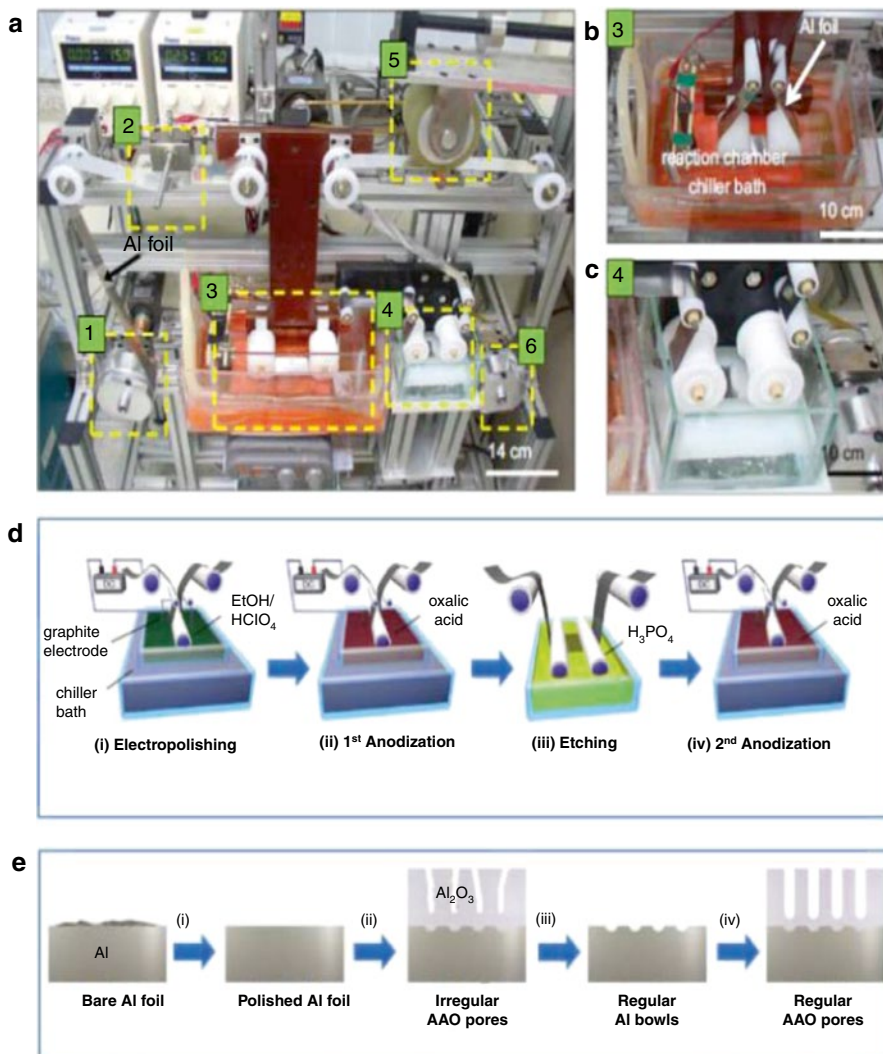
Fig. 6 R2R Al texturing system: (a) optical image of the R2R system used for Al texturization. The important components of the system are highlighted as (1) Al feeding roll, (2) electrical contact to the Al foil, (3) reaction chamber, (4) rinse bath, (5) capstan roll, and (6) rewinding roll. (b) Zoomed-in optical image of the reaction chamber, and (c) The rinse bath, respectively (d) Schematic diagrams of the process, and (e) The resulting surface structure after (i) electropolishing, (ii) first anodization, (iii) AAO wet etching and (iv) second anodization steps used for the fabrication of various surface textures (Reprinted with permission from Ref. [42] (copyright 2011, Elsevier) and Ref. [43] (copyright 2011, American Chemical Society))
