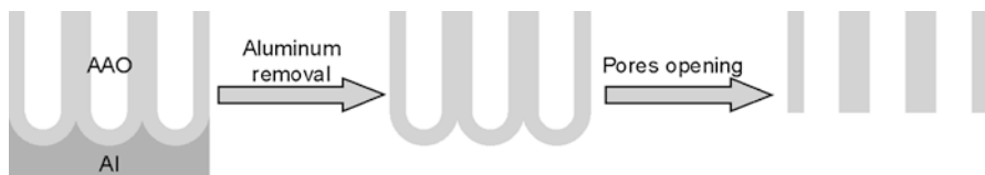
Fig. 17 Fabrication of anodic alumina templates for nanofabrication. Obtained AAO has to be detached from remaining Al, and next the pores' bottoms have to be opened (Adapted from Zaraska et al. [294])
