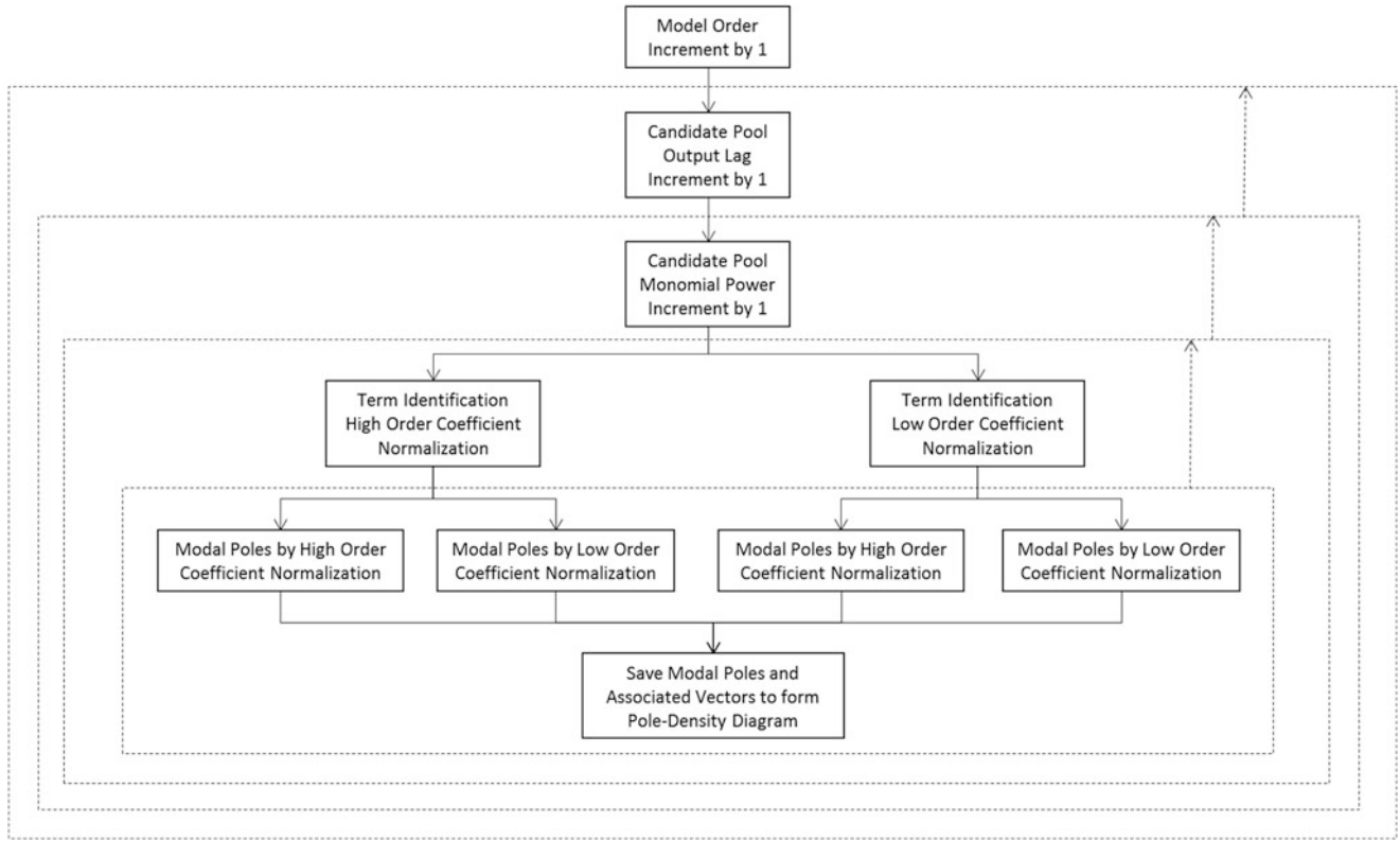
Fig. 18.1 Flowchart showing the iterations performed to generate pole-stability diagrams
