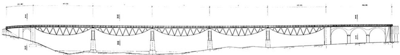
Fig. 16.2 Elevation view of E. Torroja Bridge
