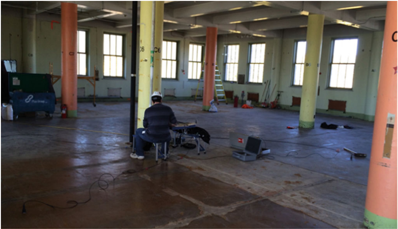
Fig. 50.2 Modal testing of Structure #1
