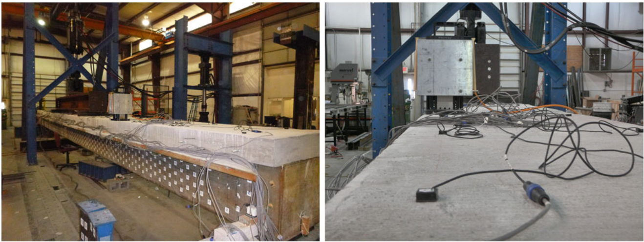
Fig. 22.4 Photographs of instrumented HCB bridge beam with reaction mass shaker and array of uniaxial accelerometers
