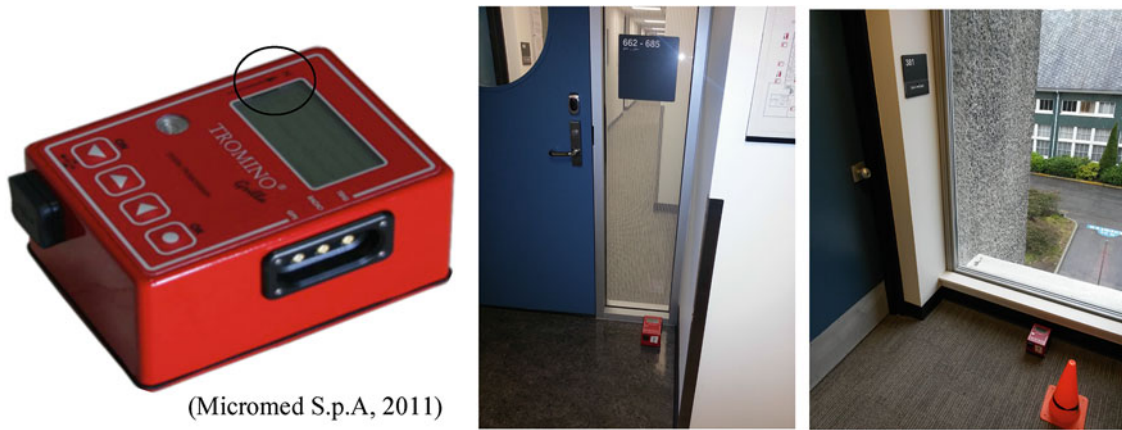
Fig. 41.5 Tromino sensor and placement locations
