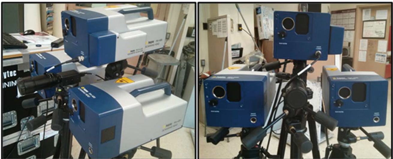
Fig. 19.1 Experimental arrangement of the 3D scanning laser Doppler vibrometer system
