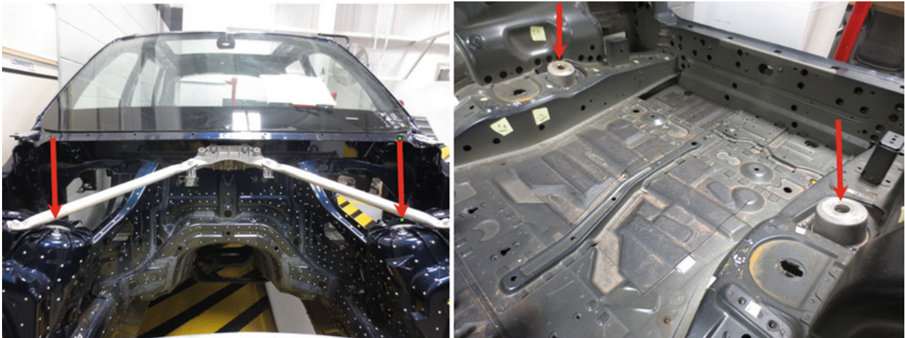
Fig. 13.5 A BMW E70 BIW showing front and rear DOF locations for eRCF measurements
