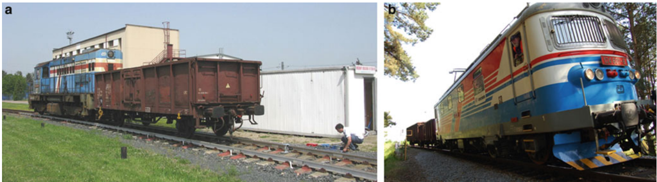
Fig. 20.5 (a) Diesel locomotive was pushing the wagon class Es into the 150 m radius curve; (b) Locomotive trailing the wagons on the 600 m radius curve
