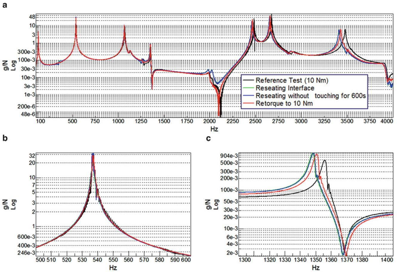
**Fig. 36.19** The FRFs of the rough interface repeatability test for (a) the entire frequency range, (b) near the second natural frequency, and (c) near the fourth natural frequency
