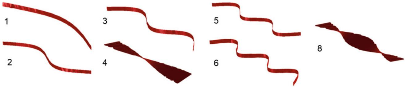
**Fig. 36.3** Mode shapes measured in modal analysis
