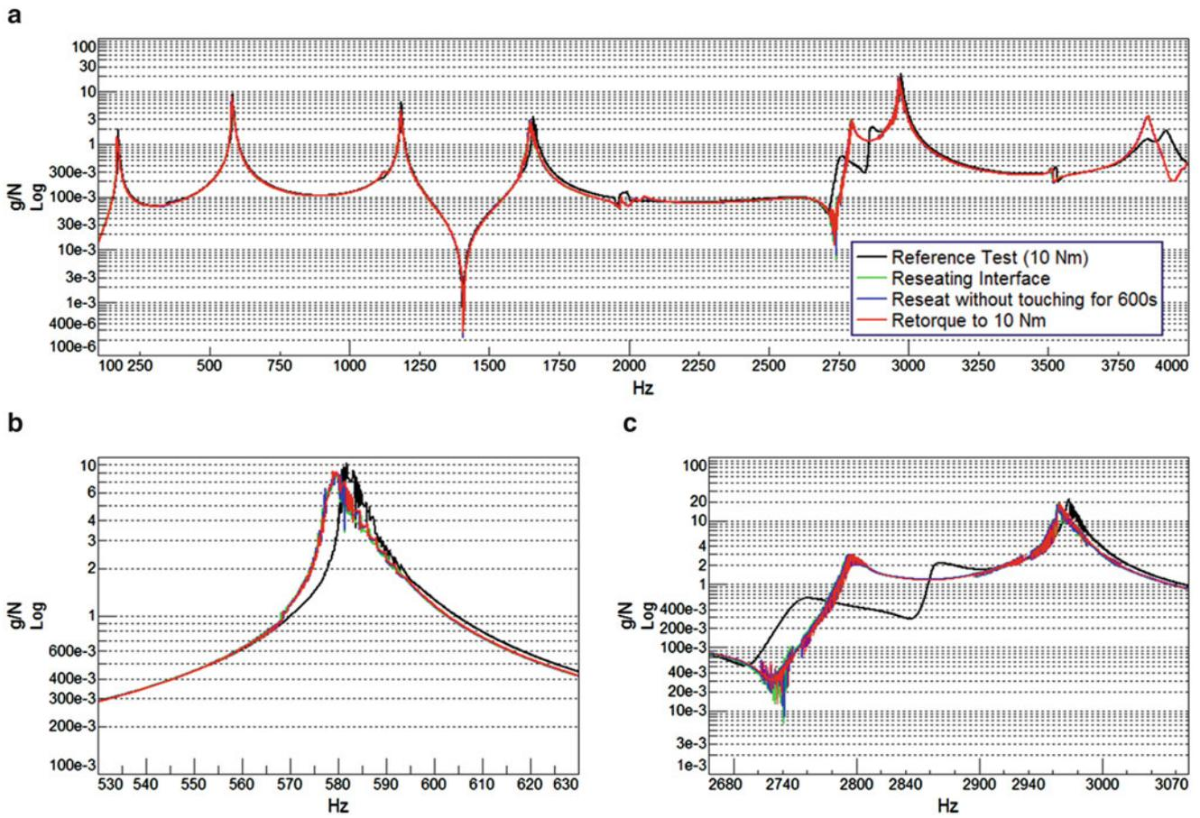
**Fig. 36.20** The FRFs of the mirror interface repeatability test for (a) the entire frequency range, (b) near the second natural frequency, and (c) near the fourth natural frequency
