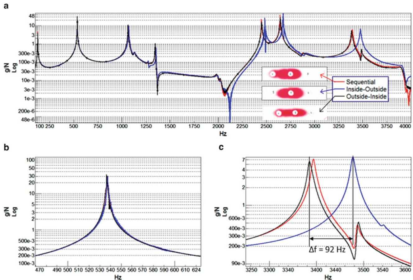
**Fig. 36.15** The FRFs of the bolt tightening order of the rough interface for (a) the entire frequency range, (b) near the second natural frequency, and (c) near the seventh natural frequency. The tightening orders are: sequential from one side to the other (*red*), the middle then the outer bolts (*blue*), and the outer then the middle bolt (*black*)
