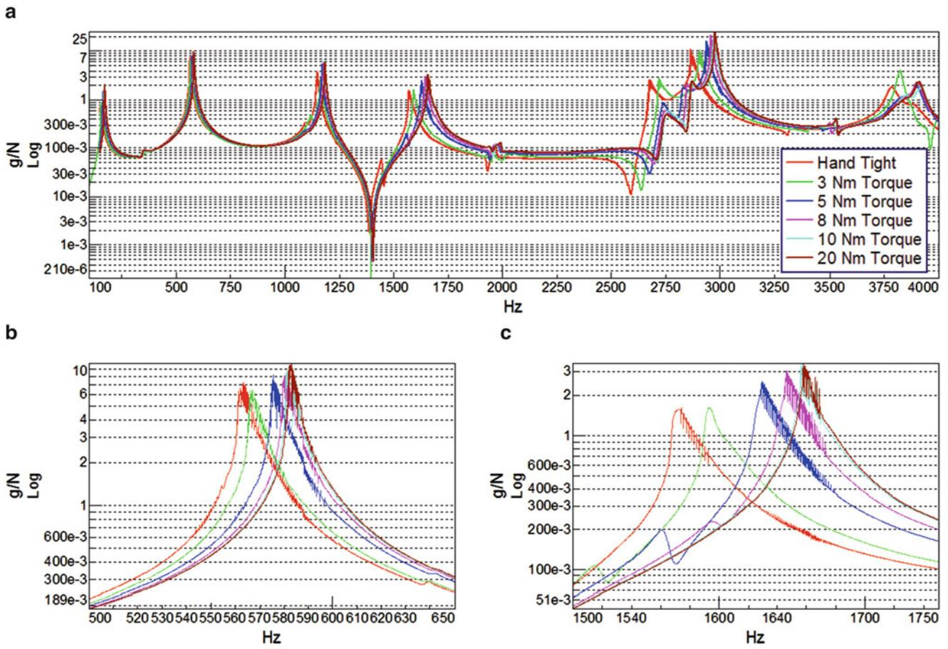
**Fig. 36.18** The FRFs of the bolt torque of the mirror interface for (a) the entire frequency range, (b) the second natural frequency, and (c) the fourth natural frequency
