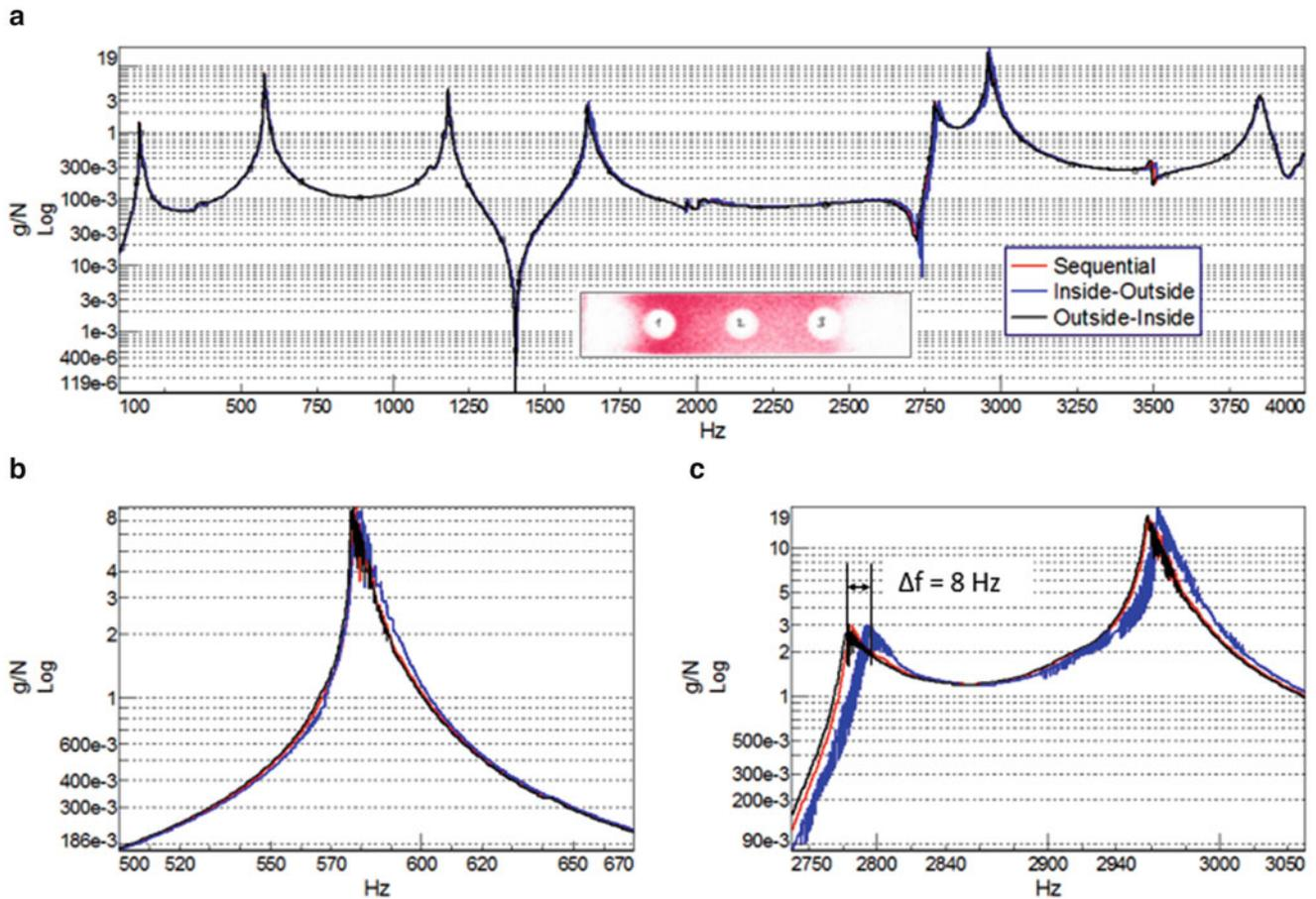
**Fig. 36.16** The FRFs of the bolt tightening order of the mirror interface for (a) the entire frequency range, (b) near the second natural frequency, and (c) near the seventh natural frequency. The tightening orders are: sequential from one side to the other (*red*), the middle then the outer bolts (*blue*), and the outer then the middle bolt (*black*)
