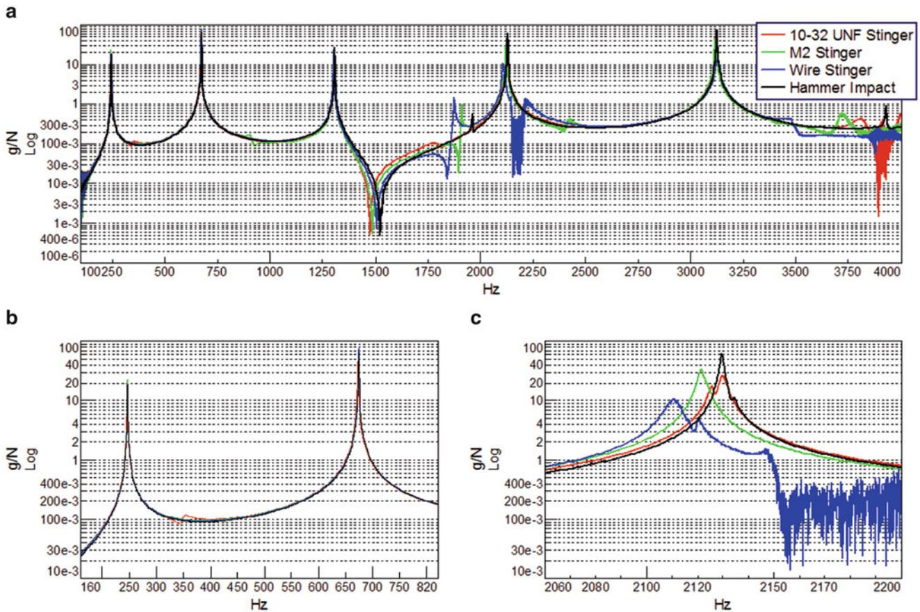
**Fig. 36.10** The FRFs of the stinger tests and one impact test for (a) the entire frequency range, (b) the first and second natural frequencies, and (c) the fourth natural frequency (as measured with the impact hammer)
