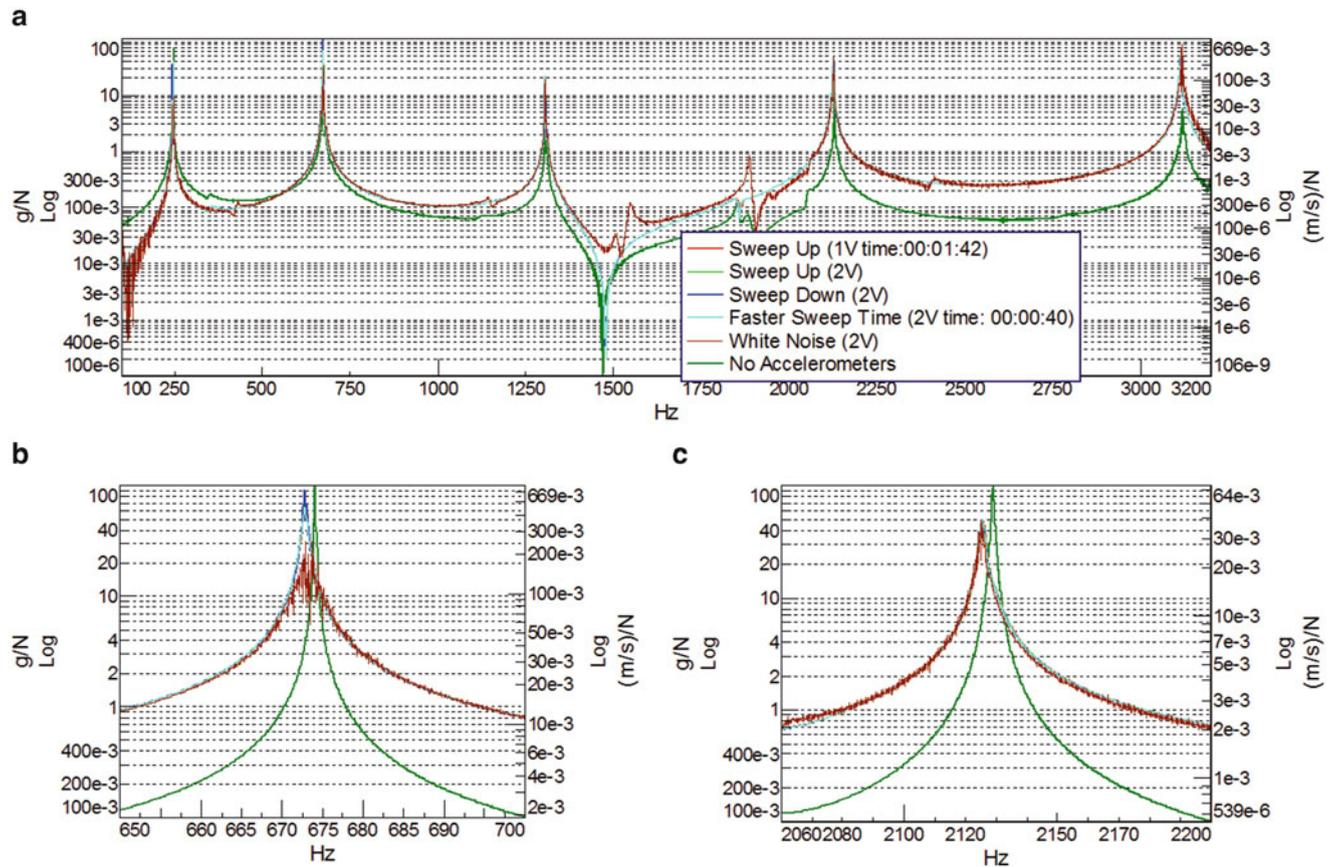
**Fig. 36.11** The FRFs of the shaker signal tests over (a) the entire frequency range, (b) near the second natural frequency, and (c) near the fourth natural frequency
