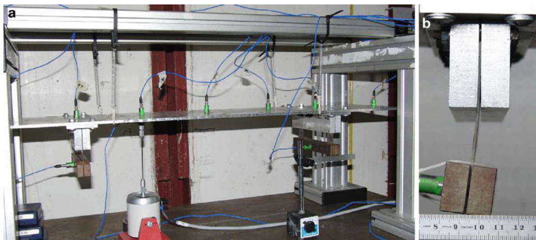
Fig. 27.1 Test structure representing the configuration of an aircraft wing having two underwing stores supported by pylons. (a) General view of the experiment setup. (b) Detailed view of the nonlinear connection
