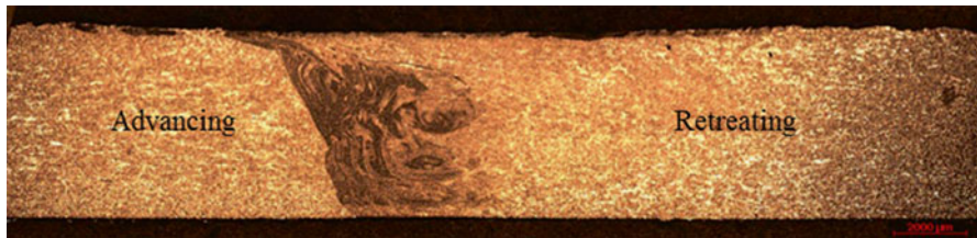
Fig. 14.1 Optical macrograph of sample 2 Al/SiC composite joined by friction stir welding
