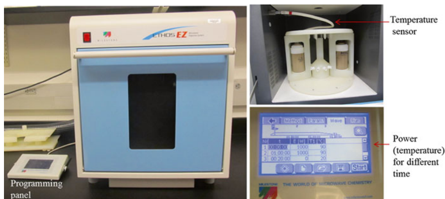
Fig. 3.5 Photograph of microwave technique ( left ), Teflon vessel (reference and material inserted) ( upper right ), and the programmed panel with power and temperature for different time. The temperature sensor is inserted inside the reference vial and provides the temperature inside the microwave system
