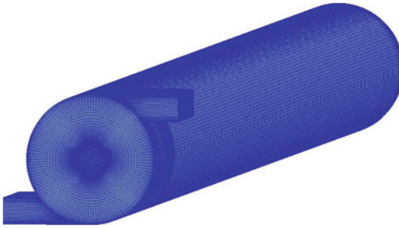
Fig. 9 Solution domain and numerical mesh
