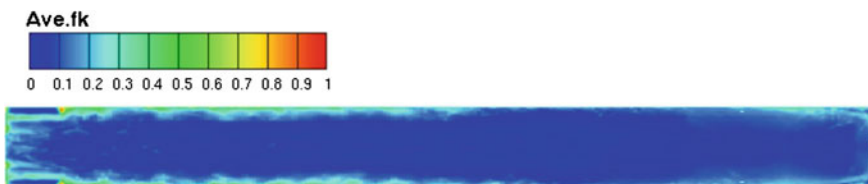
Fig. 10 Distribution of the modelled-to-total-ratio of the turbulent kinetic energy f_k
