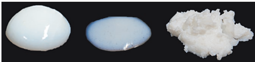
Fig. 6 Texture of aqueous dispersion ( \phi = 0.64 , R = 85 nm) without PEO ( left ) and with added PEO ( M_w = 4000 g/mol) at concentrations of c_p = 5 g/l ( middle ) and c_p = 10 g/l ( right ). Reproduced from Ref. [42] with permission
