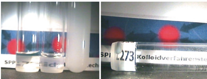
Fig. 17 Preparation of transparent highly concentrated aqueous dispersions of PFBMA-PEO particles. From left to right (i) monomodal dispersion ( R_L = 190 nm) at \phi = 0.64 ; (ii) binary mixture with \Gamma = R_S/R_L = 153 nm/190 nm = 0.805 at \phi = 0.64 —both in an isorefractive water-DMSO mixture; (iii) monomodal dispersion ( R_L = 190 nm) at \phi = 0.02 in pure water; (iv) same as (i) showing that the sample does not flow
