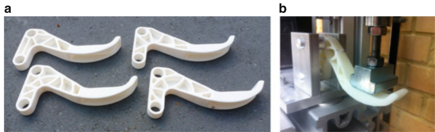
Fig. 8 The three alternative and the reference geometry have been printed using a rapid prototyping method. The right image shows the experimental setup. A load is applied and the deformation is measured until failure (a) Printed 3D geometries (b) Experimental set-up
