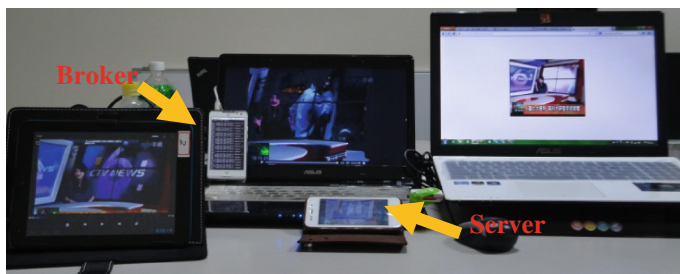
Fig. 5. In a video multicasting case, a broker is logging system operation and different types of clients are playing the same video through different physical networks.
