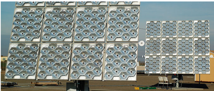
Fig. 17 SolFocus prototype HCPV system used for extracting tracker and module parameters
