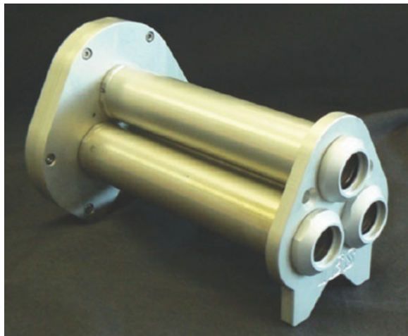
Fig. 3 Tri-band spectroheliometer based on isotype cells. Courtesy of Solar Added Value
