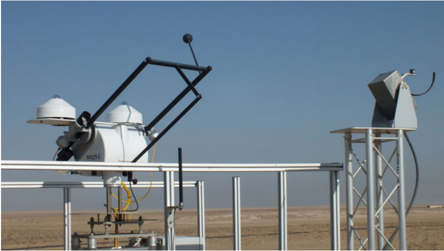
Fig. 10 Equipment for the measurement of solar radiation. To the left , a dedicated Sun tracker on which a pyrliometer and two pyranometers (shaded and unshaded) are mounted. To the right , a rotating shadowband irradiometer. Photo (c) C. A. Gueymard
