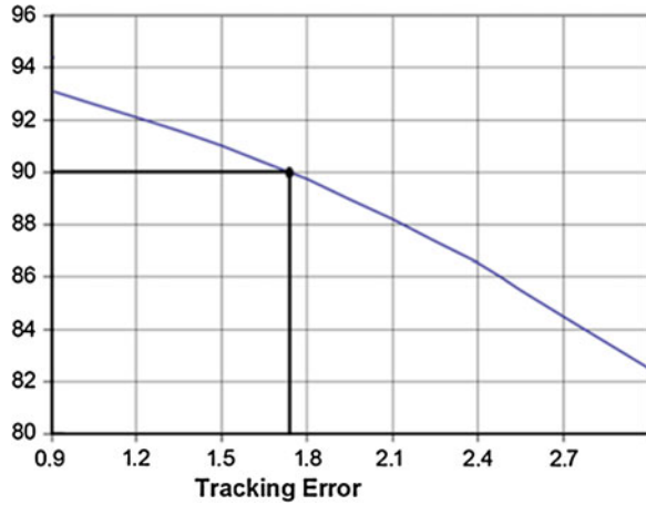
Fig. 5 Example of the variation of the module power (%) versus tracking error (°). In this case, the acceptance angle is 1.7°
