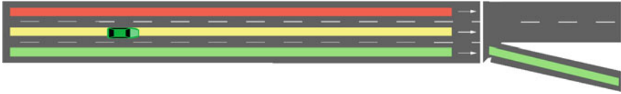
Fig. 1 The ego vehicle ( green ) needs to move to the bottom lane (with index 0) in order continue on its desired route ( green ). This lane has a bestLaneOffset of 0. The yellow lane (with index 1) has a bestLaneOffset of -1 indicating a necessary lane change to the right. The red lane (with index 2) has a bestLaneOffset of -2 and is strategically unadvisable
