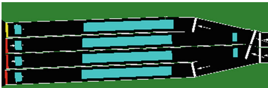
Fig. 2 Typical detection field for vehicle actuated control
