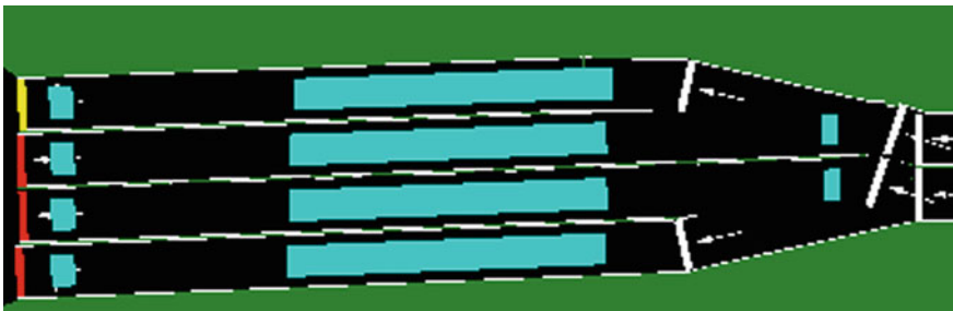
Fig. 2 Typical detection field for vehicle actuated control
