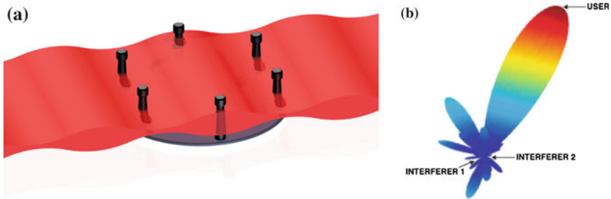
Fig. 15.2 a An antenna array uses phase information to detect the direction of arrival of an incident wave. b Adaptive array coverage: a representative depiction of a main lobe extending toward a user with null directed toward two co-channel interferers [3]
