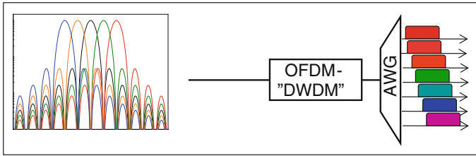
Fig. 9.13 Reception of OFDM signals using a WDM-type receiver requires an OFDM-to-“DWDM” data format conversion. This may be achieved with a spectral telescope
