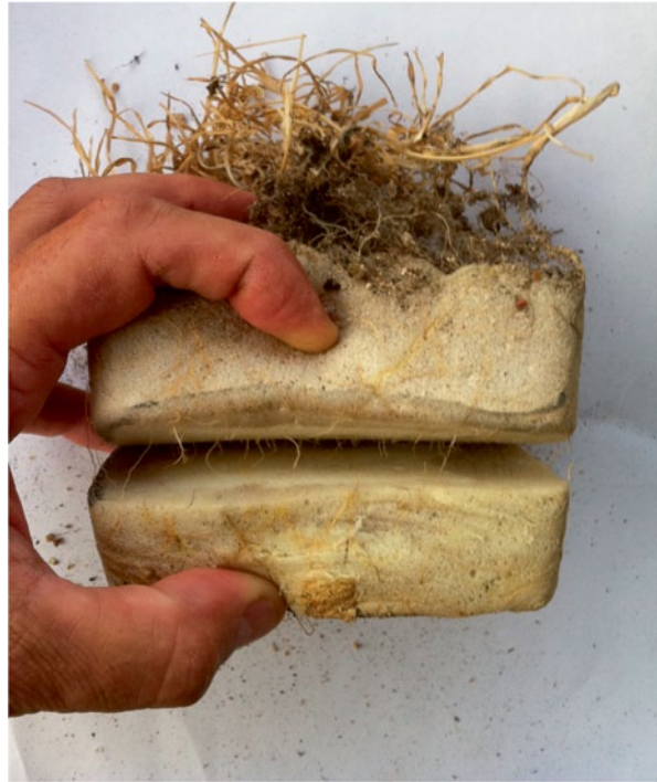
Fig. 3.2 Experimental hydroponic foam layer used beneath the growing media to accommodate both stormwater retention and providing plant available water Note the roots both above and penetrating through foam layers ( Mark Simmons )
