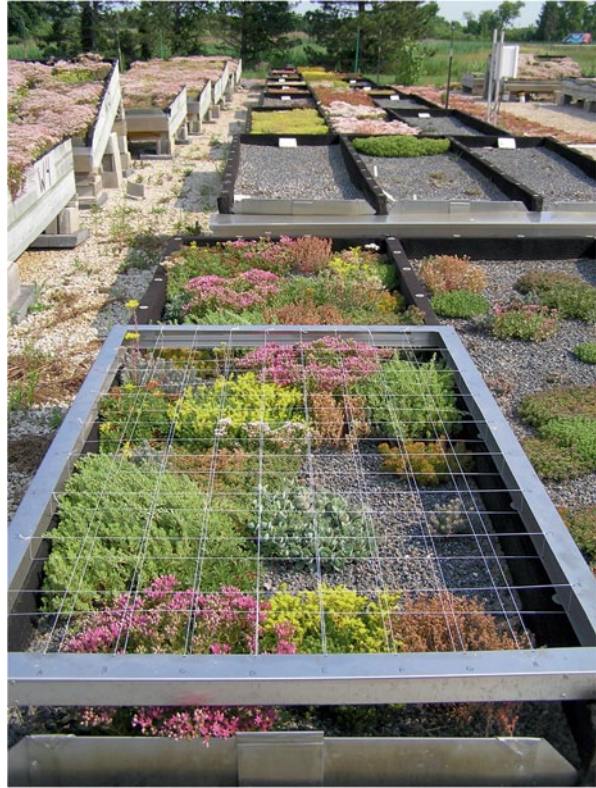
Fig. 13.2 Use of a point frame to measure absolute cover on the Horticulture Teaching and Research Center green roof at Michigan State University. (Photo DB Rowe)
