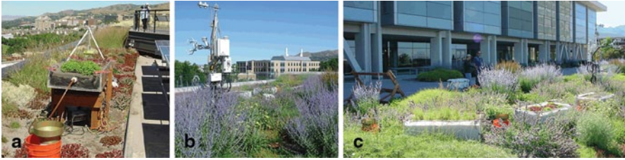
Fig. 2.8 Green roof monitoring setup on two roofs in Salt Lake City, Utah: (a) Natural History Museum of Utah; (b) and (c) University of Utah J. Willard Marriott Library (Lee R. Skabelund)
