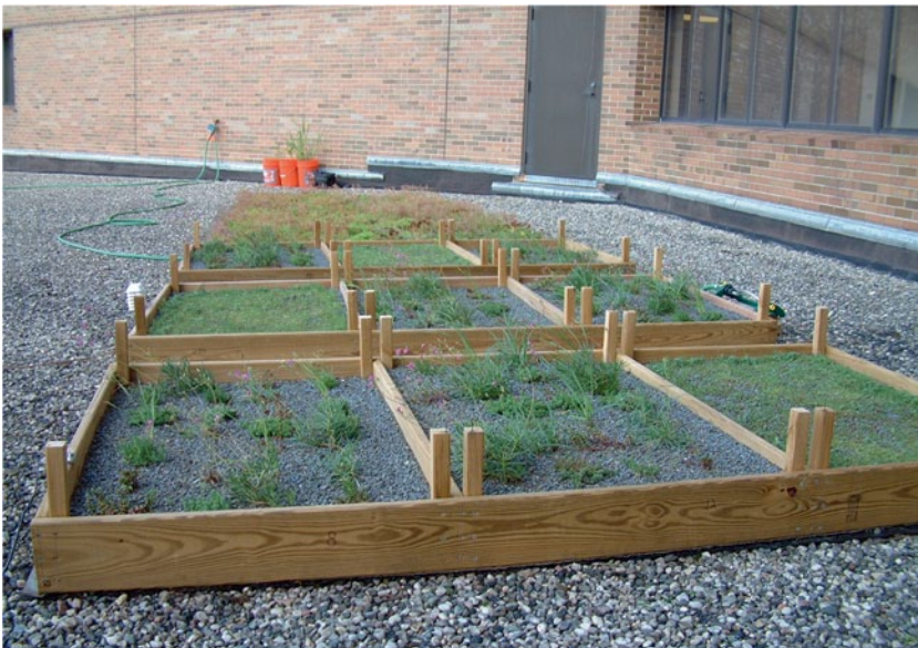
Fig. 13.1 Replicated research plots located in the shade on the Communication Arts and Sciences Building at Michigan State University. (Photo DB Rowe)
