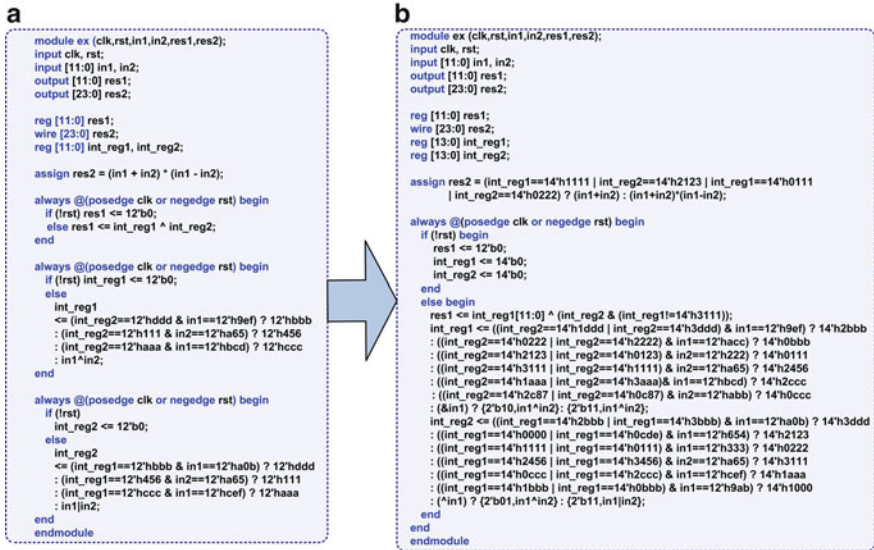
Fig. 10 Example of RTL obfuscation by CFG modification: (a) original RTL; (b) obfuscated RTL [12]
