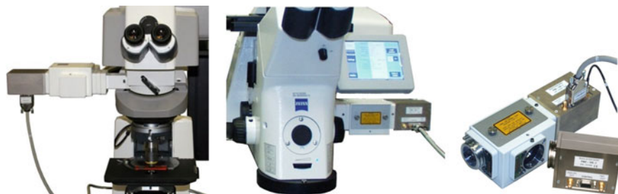
Fig. 2.8 NDD detection at the LSM 710. Left Upright microscope. Middle Inverted microscope. Right NDD beamsplitter cube for two FLIM detectors. The 90° output is shown with the detector de-attached
