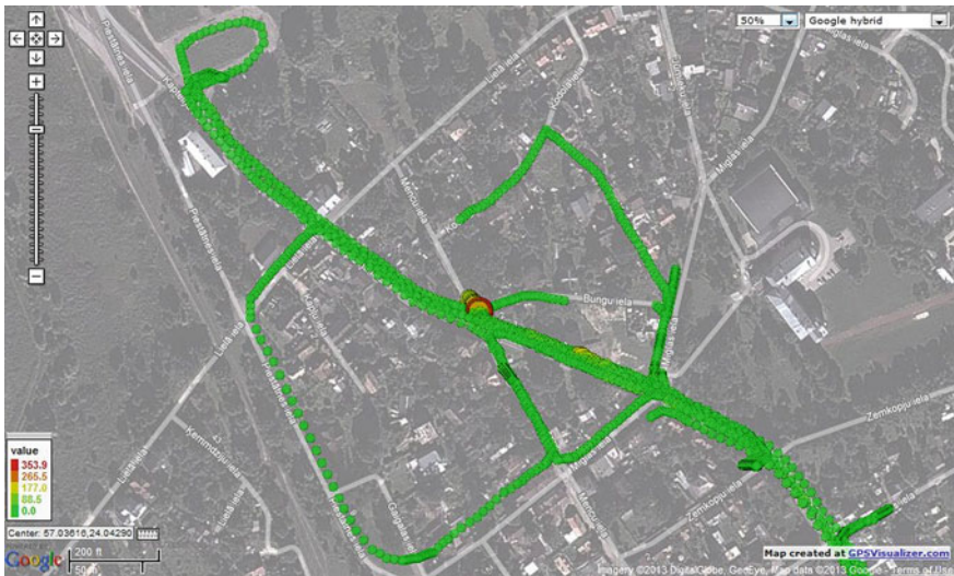
Fig. 6 Map-projected mercury concentration in air on Gobas street (May 2, 2012, registered from drive-by car)
