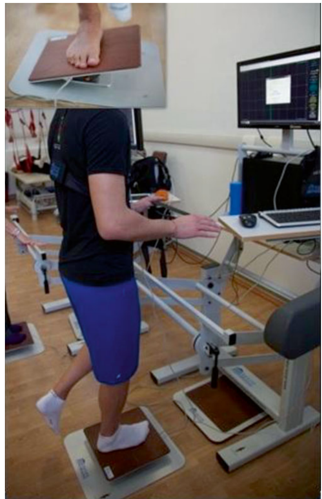
Fig. 54.3 Electronic postural proprioceptive station (Delos Postural Proprioceptive System, Delos, Torino, Italy). You can see the activity of the patient records on charts
