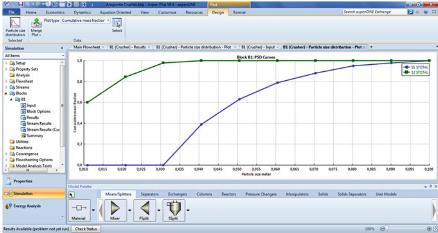
Fig. 9.13 PSD from inlet and outlet streams for aragonite crusher example in Aspen Plus ®
